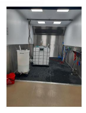
DRUM Wash Systems : 2 drums – 1 IBC - a HIGH PRESSURE PUMP
