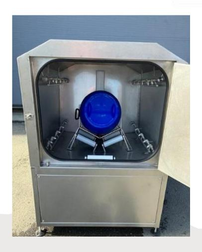
This is an automated wash system, high pressure low flow, a very efficient wash
